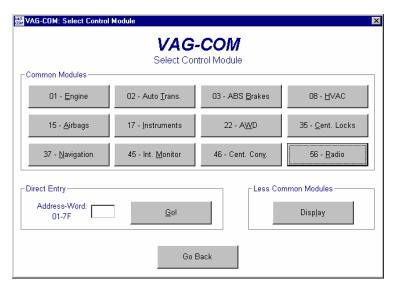
Next return to the Select Control Module and select 37 – Navigation (Note if you have the TV tuner it's Control Module 57)
