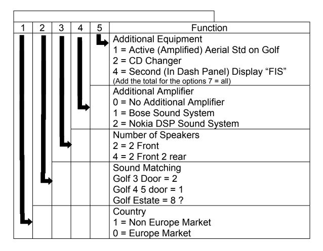
Therefore 01417 is a Navigation system fitted to a European 5 door Golf, with Bose Sound System, CD changer, active aerial and FIS display
