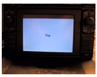
The radio will go off and the screen will display "Diag", in addition if you have an instrument cluster display this will also display "Diag". You may hear the odd click from the speakers, this is normal and is caused by the unit checking the connection of the speakers.
