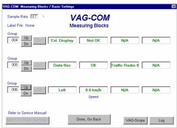
The Measurement blocks for the Navigation side are self explanatory, Group 002, reverse is as it says, if you select reverse gear is goes to Reverse ON, terminal 15 is the ignition ON.
