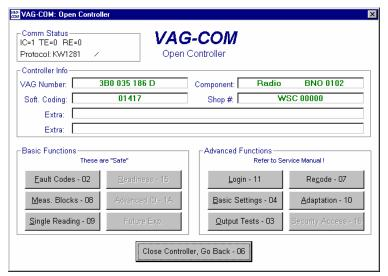
The item of interest on this screen is the Soft Code use the table below to set the Soft code using the Recode-07 function
